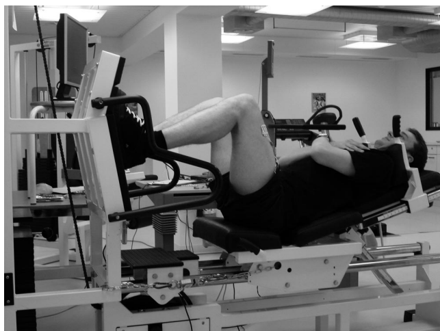
Fig. 2. The horizontal leg press machine equipped with the strain gauge.
